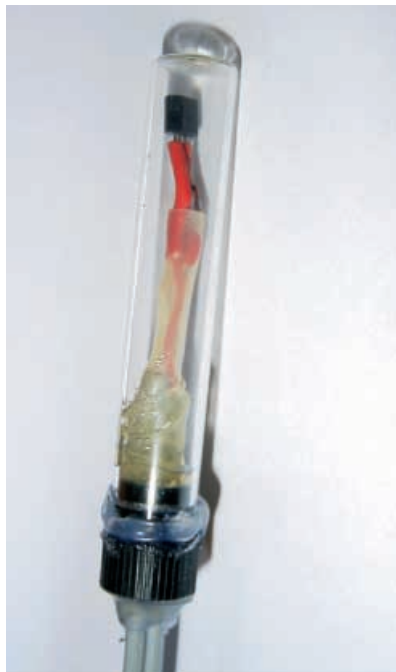
The LM35DZ enclosed in a sealed glass tube.
