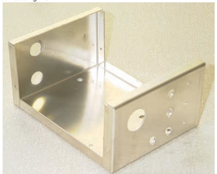
The aluminium chassis drilled for the front and rear panel mounting components. Use the transformer and circuit board as a template to mark the drilling positions on the base of the case.
