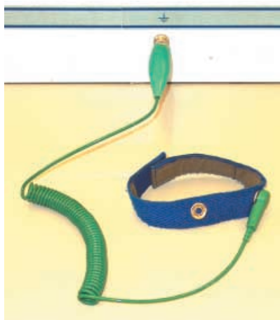
Photo 4.1. An earthed wrist strap which prevents the build-up of static electricity in the user.
