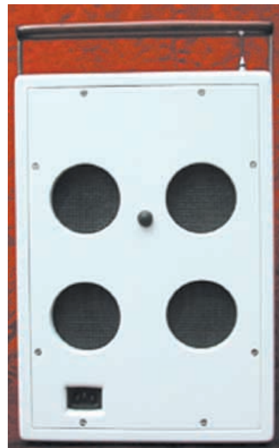
Rear panel showing the four speaker vent holes. These holes also ensure adequate airflow to cool the transformer and heatsink.
