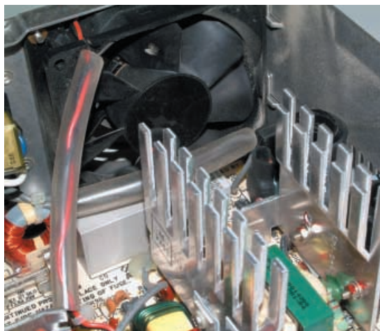
Internal view of a power supply that uses fan cooling to draw cooler air over a heatsink.
