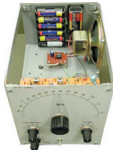
The two separate power supply battery "packs", one for the receiver and the other for the amplifier, located on the rear panel.
