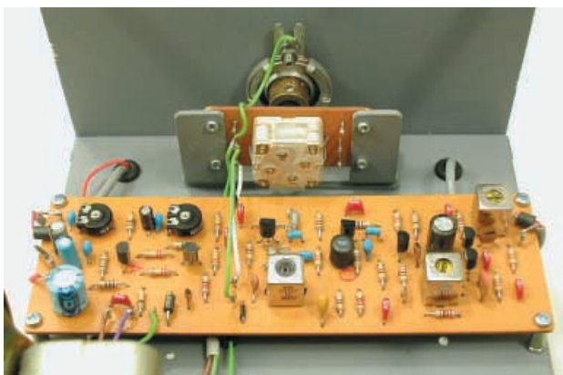
Receiver p.c.b. mounted on the metal chassis and wired to the tuning capacitor board.
