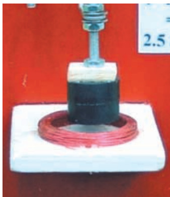
Fig.6. Making the coil former. For the dotted piece A5 see the text. The completed coil is shown in the photograph.
