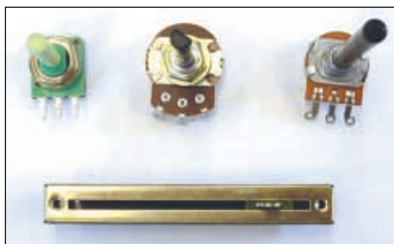
Photo 1.2. Example of panel mounting single potentiometers.
