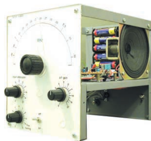
Completed 7MHz version of the Direct Conversion Receiver. If a 3-Band version is to be built, the band change rotary switch is mounted in the blanked-out hole just below the tuning knob.
