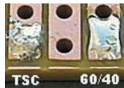
Fig.2. Comparing TSC lead-free solder to standard 60/40.
