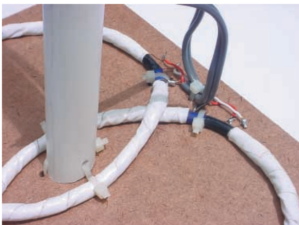
Close-up of the search head showing the cable ties securing the shaft "handle" to the plate.
