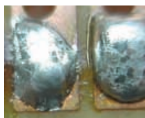
Fig.5. Lead contamination seen as a mottled surface.
