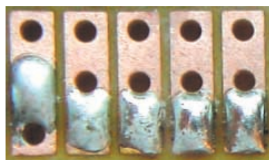
Fig.6. Effect of diminishing lead content.
