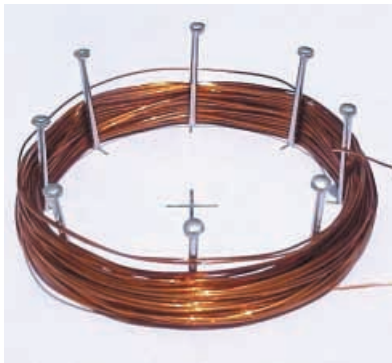
Enamelled copper wire (30s.w.g.) wound around the guide pins.
