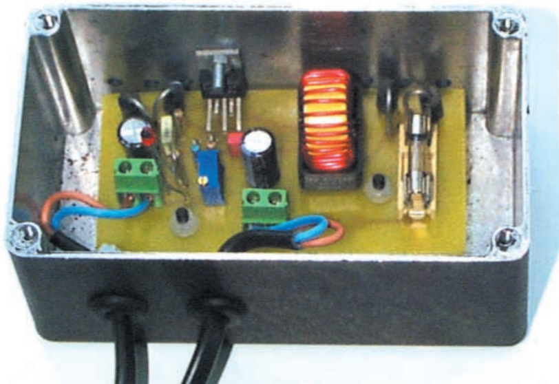
Finished power supply showing the p.c.b. mounted in a diecast box.
