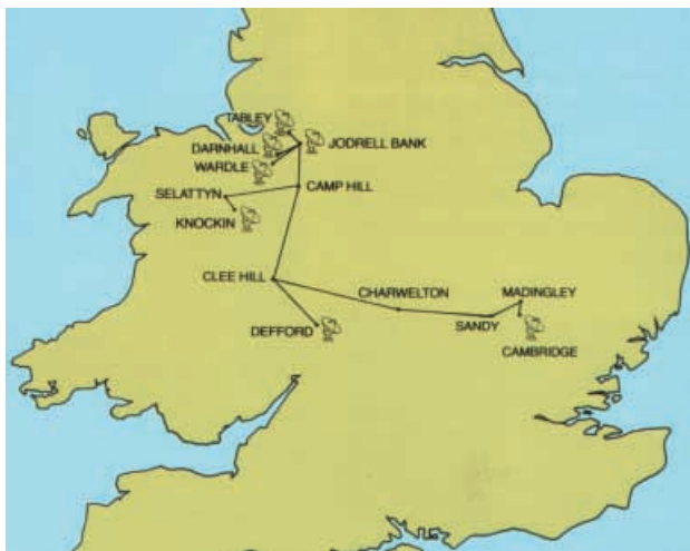
Fig.9. The Merlyn array of radio telescopes and repeater stations showing the microwave links to Jodrell Bank.
