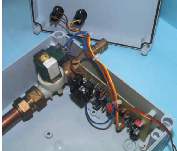
The low-voltage d.c. solenoid water valve unit mounted in one corner of the waterproof case.
