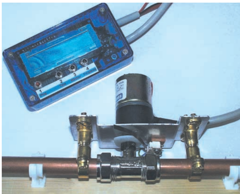
Completed PIC Watering Timer controller together with "plumbed-in", motor driven, water valve.
