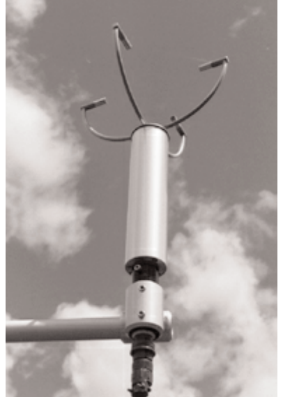
CAT1/2 solid-state ultrasonic wind speed and direction sensor. Photo Courtesy www.apptech.com/cat12.htm , Applied Technologies, Inc.
