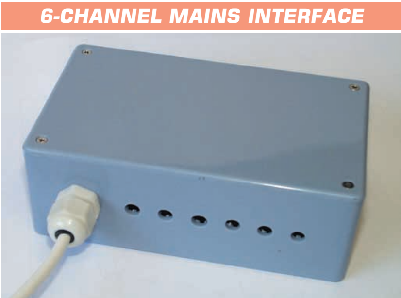
Completed Interface unit. The six holes for the mains output leads to the lamps must have lead clamping grommets mounted in them.
