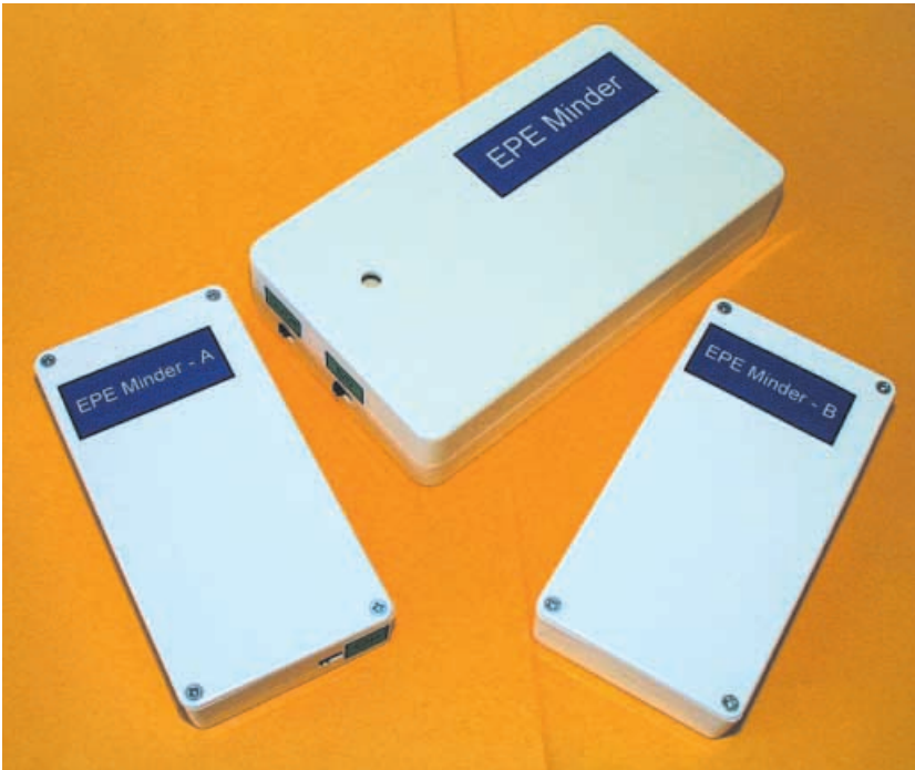
EPE Minder Receiver (top) and two Transmitter units. These models incorporate type-approved, pre-aligned, 433MHz transmitter and receiver modules. No operating licence is required in the UK.
