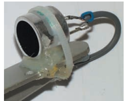
Transducer secured to probe mount using a cable tie and hot-melt glue.
