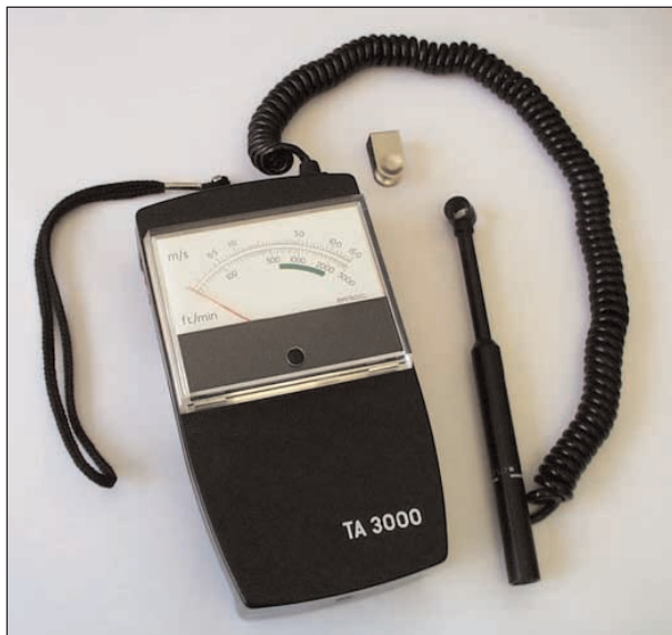
Commercial thermal anemometer lent to the author by Andy Flind.
