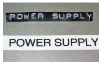
Fig.2. The label from the Dymo Mini (top) is not as good as one from an electronic labelling machine (bottom). Results are adequate though, and can be improved if due care is taken when stamping the letters and handling the tapes
