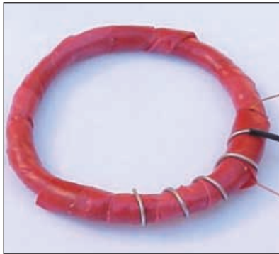
Taped-up coil and the Faraday shield connecting wire
