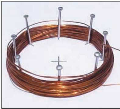
Enamelled copper wire (30s.w.g.) wound around guide pins (former)
