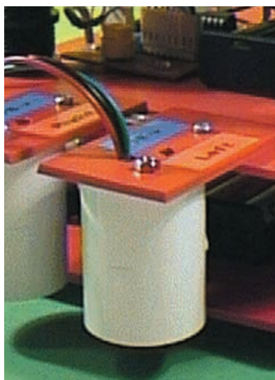
Close-up of one of the two, front-mounted, infra-red line sensors.
