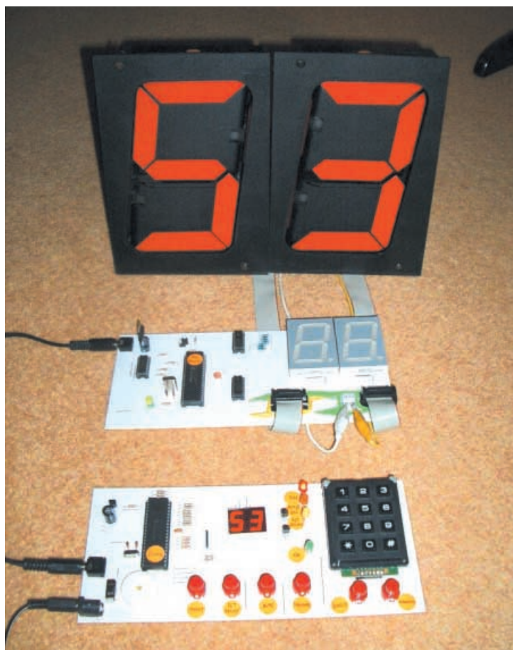
Two large “big-digit” mechanical 7-segment displays connected to the volt-display interface board, which is also linked to the main Bingo Box p.c.b. a g e
