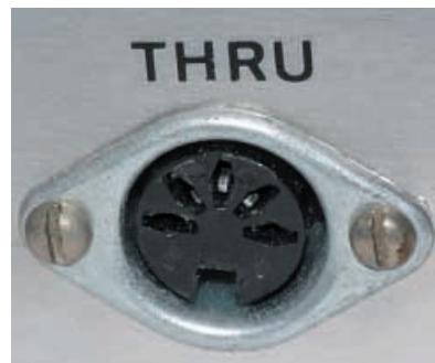
Fig.5. A chassis mounting DIN socket requires a main 12.5mm mounting hole and two smaller holes for the 6BA or M3 mounting bolts.
