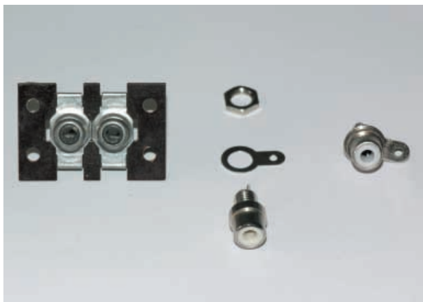
Fig.3. Phono sockets. Old style dual socket (left), disassembled single socket (middle), and assembled single socket (right).
