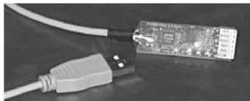
FEDPIC Key – Ultra-Miniature USB In Circuit Serial Programmer and Debugger
