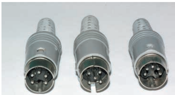
Fig.4. The range of DIN connectors is vast. These are all 5-way DIN plugs. From left to right they are 240°, "Domino", and 180° plugs.
