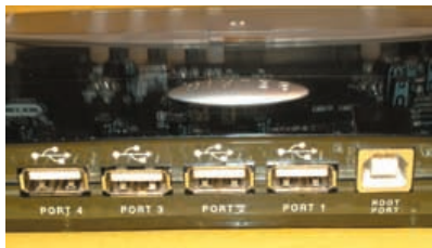
A USB hub showing four ports plus the B-type connector
