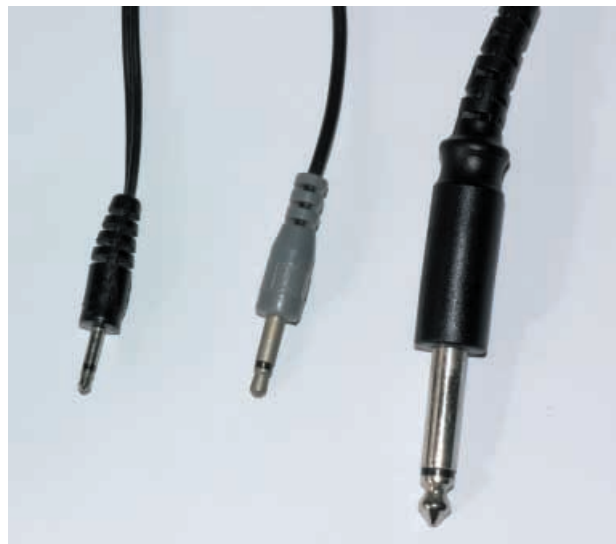
Fig.1. The miniature jack plugs (middle and left) are much smaller than the standard type (right).
