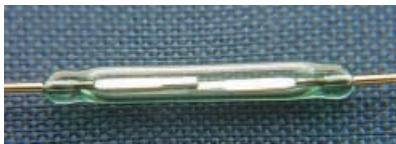
Typical glass-encapsulated reed switch, with normally open contacts
