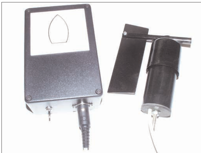
The electronic control box and vane/encoder masthead assembly.
