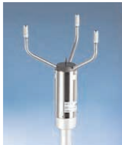
Fig.2. An ultrasonic wind sensor.
