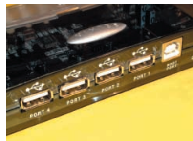
A USB hub showing four ports plus the B-type connector.
