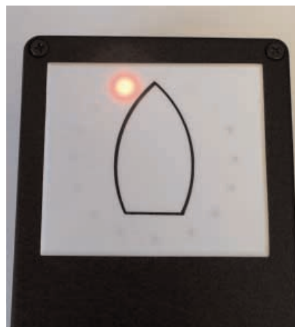
An l.e.d. showing through the sub-panel.
