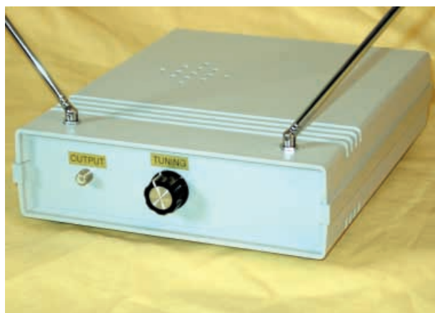
Rear view of the Theremin showing the phono output socket, tuning control (VR4) and sensor "aerials" mounting.
