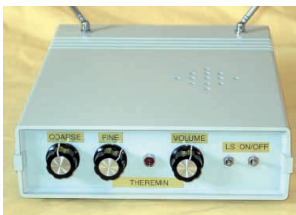
Front view showing layout of the most used controls. The loudspeaker is glued to the underside of the top panel.
