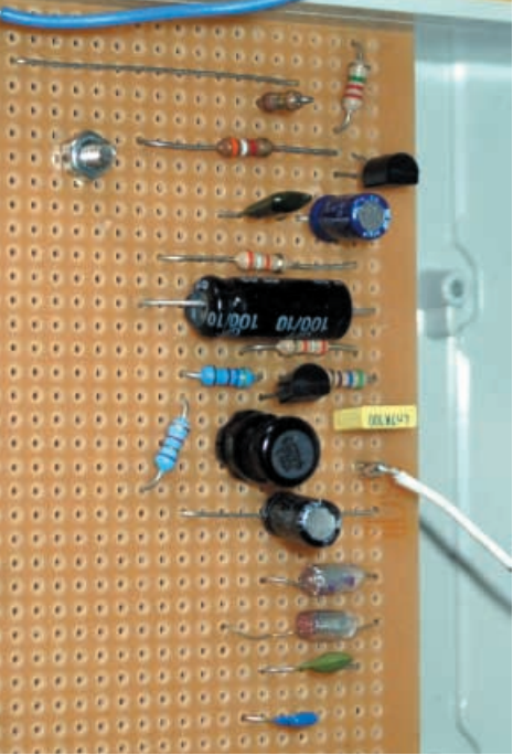
Top-left of the circuit board showing component layout for the tone generator.
