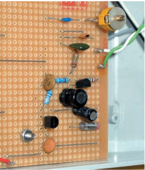
Top-right corner of the circuit board showing layout of components for the "tuneable" oscillator, including the miniature trimmer capacitor.
