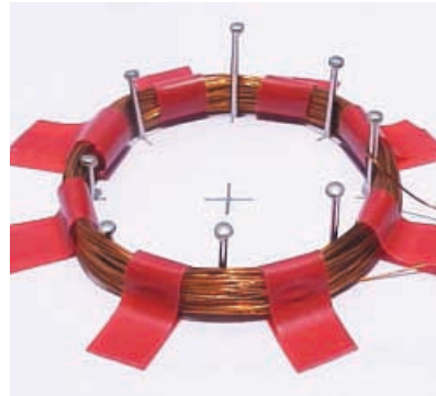
Strips of insulating tape used to hold coil windings together.
