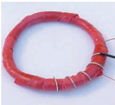
Taped-up coil and start of the Faraday shield; bared wire.
