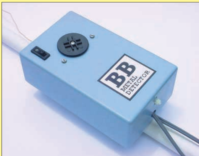
Completed detector unit showing the Sensitivity control knob (disc), on/off switch and search head cable entry.
