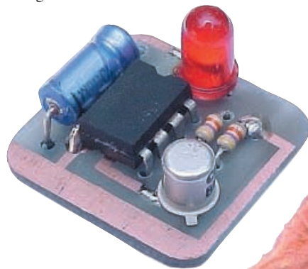
Components mounted on the topside of the completed p.c.b. Note that the junction of IC1 pin 8 and resistor R2 is soldered on both sides of the p.c.b.
