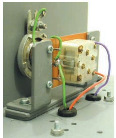
Above: Chassis view of tuning capacitor mounting, which is mounted directly above the p.c.b.
