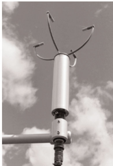
CAT1/2 solid-state ultrasonic wind speed and direction sensor. Photo Courtesy www.apptech.com/cat12.htm , Applied Technologies, Inc.
