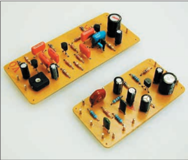
Bandpass Filter (top) and Tone Control p.c.b.s.
