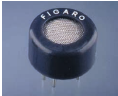
Example of a gas sensor from Figaro.
