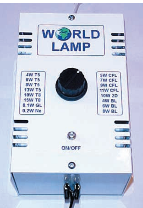
Completed World Lamp in a robust well-ventilated metal case.
