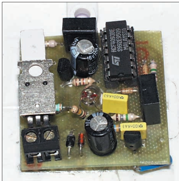
Completed circuit board. Note the neon has been bent over to lie directly over the centre hole in the p.c.b.
