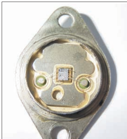
A TO-3 can style regulator sawn off to reveal the i.c. chip inside.
