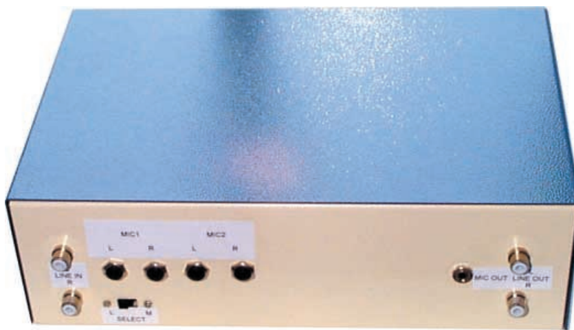
Rear view of completed unit showing positioning of the jack and phono sockets. Also shown is the output select switch.
