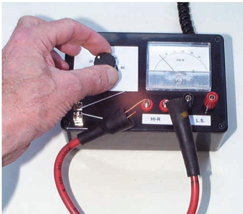
Testing an ignition (plug) lead. The new meter scaling can also be seen here.
