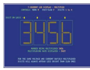
Photo 12.4. Screen dump of the interactive 4-digit l.e.d. display being multiplexed at a fast rate, all digits appear visible.
