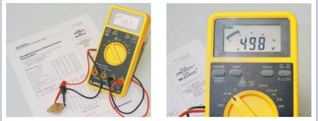
The diode test range of a digital multimeter can be used to measure the forward voltage of a transistor diode. A good reading is in the region of 0.45V to 0.9V.
