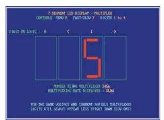
Photo 12.5. Screen dump of the interactive 4-digit I.e.d. display being multiplexed at a slow rate, only one digit is seen at a time.
