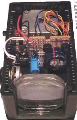
Close-up view of the "beam window" showing the lenses slotted into p.c.b. retaining guide slots. The circuit board is positioned further back in the slots, see photograph below.
