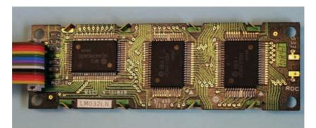
Photo 12.8. Control electronics on the rear of a 2-line by 20 (per line) character alphanumeric l.c.d., with 1400 pixels. It can be externally controlled by just six connections (plus power lines).
