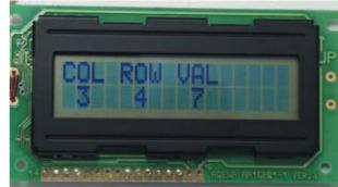
Photo 12.7. Typical alphanumeric l.c.d. screen. This one has two lines, each of 16 character cells.
