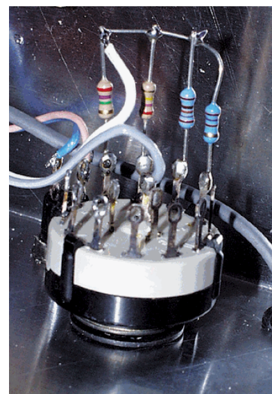
Fig.4. Camera Shutter Timer stripboard component layout, inter-wiring and details of breaks required in the underside copper strips. (Right) Mounting the Range resistors directly on the switch tags before it is fitted in the case will help with the final wiring.
