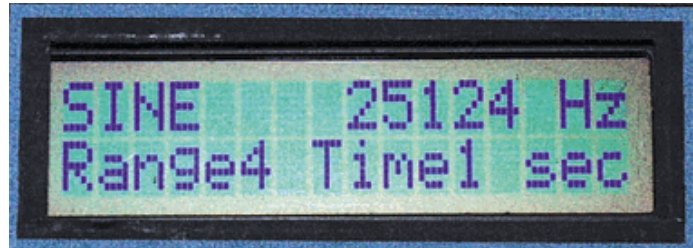
This display shows a sine wave is being generated and a frequency of 25,124Hz has been registered via range 4.
