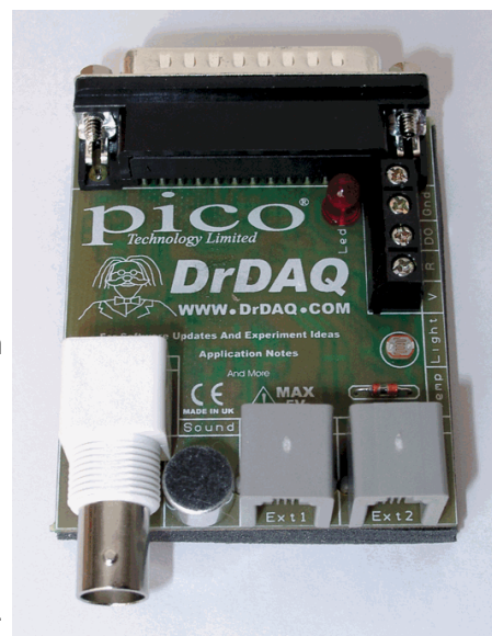
Fig.2. The uncased DrDAQ circuit board showing the parallel port connector, three sockets plus microphone. The underside components are hidden by a
