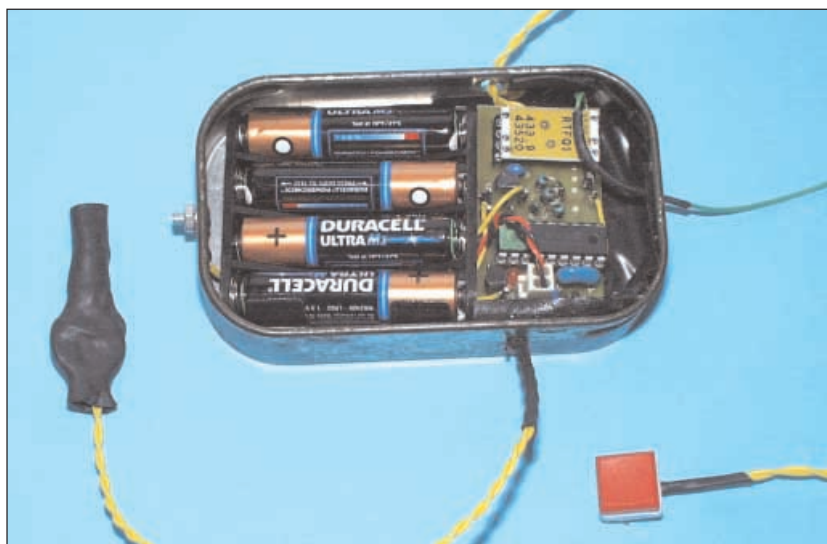
Component positioning inside the prototype transmitter's metal case. A trembler motor, encased in heat shrink sleeving, is shown on the left and a "toe/foot" switch on the right.
