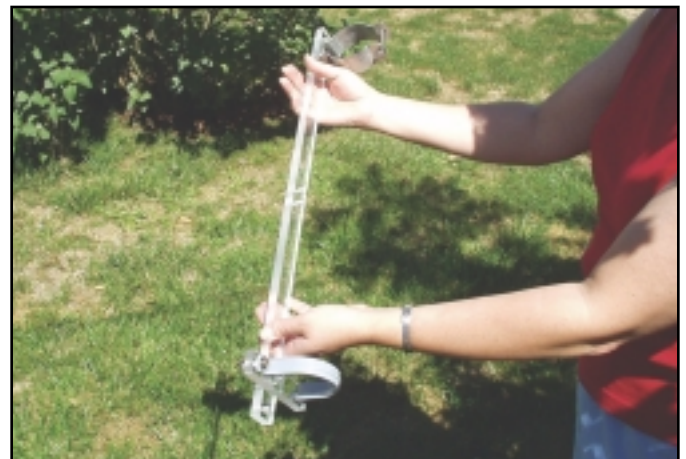
The antenna's balun and balancing network fasten to this part of the Barker & Williamson mounting kit.
