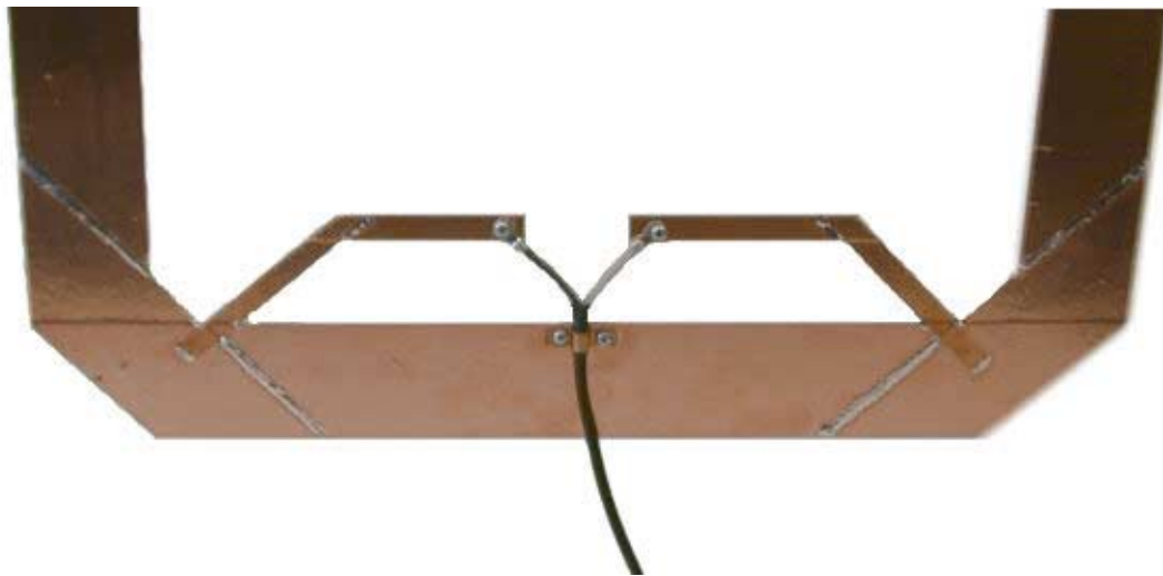
Figure 18. T-Matched Tape Antenna
