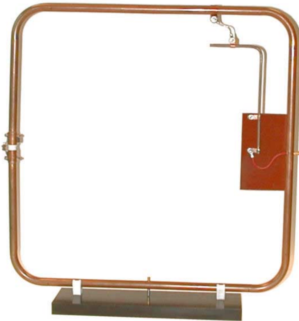
Figure 14. Gamma Matched Antenna
