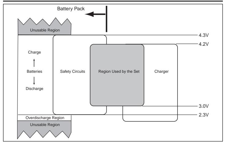
The safety circuits in the diagram above are for overcharging, overdischarging, and overcurrent for a single cell battery pack. Please contact Panasonic when two or more cells are connected or when actually using this or other circuits.
