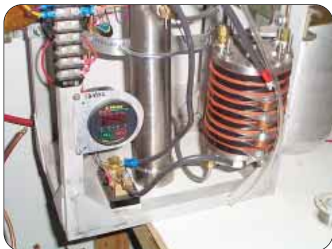
The PEM electrolyzer stack—eight cells operating at 2 VDC nominal per cell—separates the hydrogen and oxygen atoms of water molecules.
