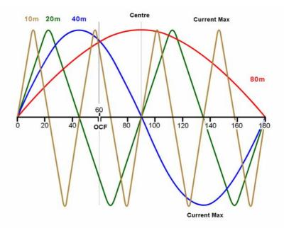
Figure 3. - A Half wavelength antenna fed at 60 degrees
