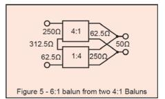
A transmission line balun designed for the impedance ratio 100:25 would not work as well (if at all) in a network with 200 and 50 Ohm impedances even though the ratio is the same.
