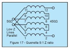
Now figure 17 does look a bit complicated but please take the time to have a good look at it. Recall how the 4:1 balun was simply two 100 ohm transmission lines on a toroid. Series connected on one side to give 50 Ohms and parallel connected on the other to give 200 Ohms.
