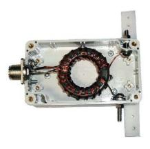
Figure 13 – The mounted 4:1 Balun – consider using eye bolts instead of the backing board.
