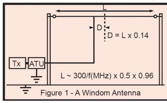
There is <u>no transmission line</u> used on the original Windom. A single wire is attached 14% off the centre of the dipole. This wire feeder is then connected to an antenna tuning unit (ATU). The idea of feeding the half wave off centre was to find a point where the
