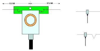
Figure 14 – Antenna dimensions
