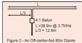
**Note**: When on 80 metres I operate usually much lower down than 3.7 MHz and in fact the SWR is very flat even if you vary these dimensions by 2-400 mm. I have found that a good, neat, and easy to remember size for an 80 metre OCF is <u>27 metres one side and 13.5 metres the other</u>. I use 1.25mm galvanised iron wire because it cheap, strong, hard to see and is stretch resistant. However you can use any wire that you like.
