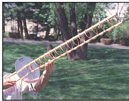
Most communication with space, both manned shuttles and unmanned satellites, uses VHF, UHF or microwave frequencies. This homebrewed antenna was designed to be used for a new satellite called Phase 3D .
