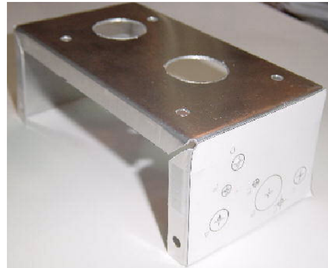
Figure 2. Using a template for drilling
