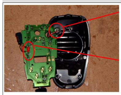
Remove the electret microphone capsule and remove their black foam in front of the capsule. Also remove the additional black foam in the mic hole of the mic front.
