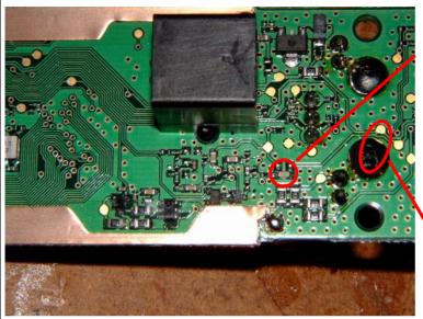
Solder a  $0.47\mu F$  electrolyt capacitor parallel C2062 (5,6nF) on the Panel-Unit.
