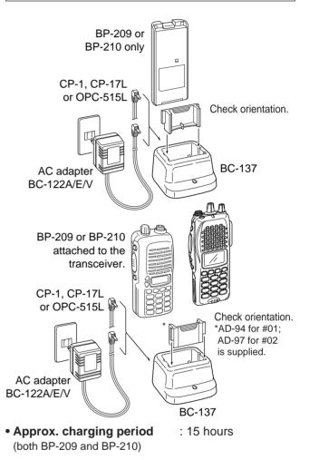
Batteries MUST BE removed from the BC-137 to stop charging. Kenne 15 hours of charging. stop charging. Remove BP-209 or BP-210 after
